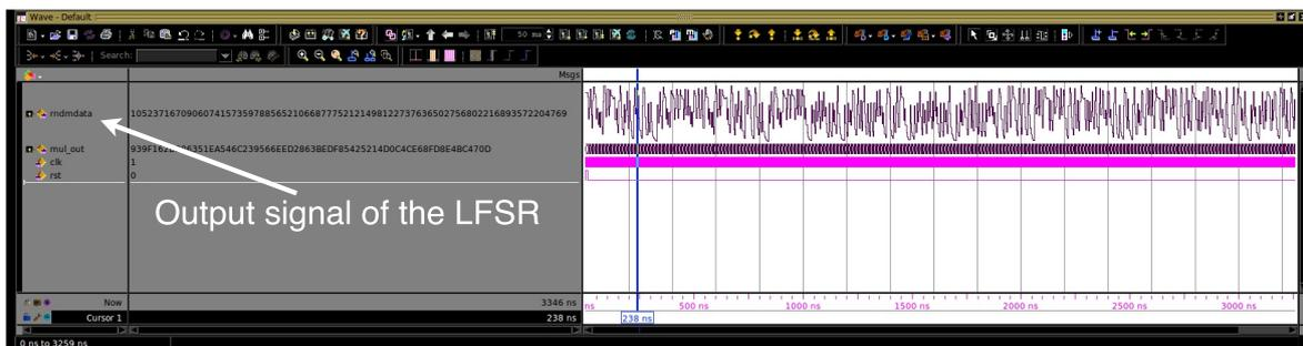
Figure 10: Randomness of the data generator based on a 256-bits LFSR.
