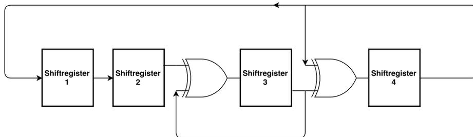
Figure 6: A 4 bit Linear Feedback Shift Register (LFSR)
