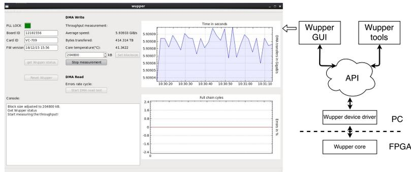
Figure 7: High and low level software overview block diagram.
