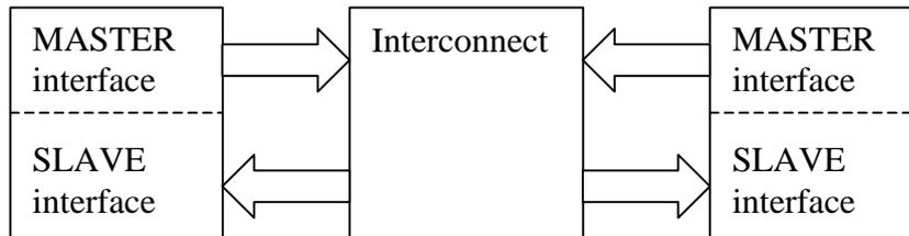
In large designs these additional interconnect signals could cause routing problems. If the increased bandwidth is not needed than a substantial reduction in the number of interconnect signals can be achieved by combining common signals between MASTER and SLAVE interfaces.
