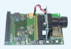
For autonomous robots, various sensor capabilities are crucial. The GECKO3sensors board therefore houses a variety of sensors like a two-dimensional magnetic field sensor for compass application, a two-dimensional acceleration sensor, digital video camera for image processing as well as a bluetooth wireless communication device.
