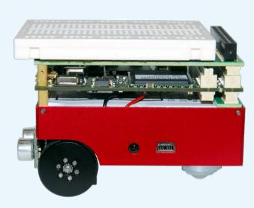
The GECKO system is a general purpose hardware/software co-design environment for real-time information processing and/or system-on-chip (SoC) solutions. The GECKO system supports a new design methodology for system-on-chips, which necessitates co-design of software, fast hardware and dedicated real-time signal processing hardware.
