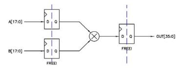
Figure 13. Signed multiplier hardware typically found in an FPGA.
