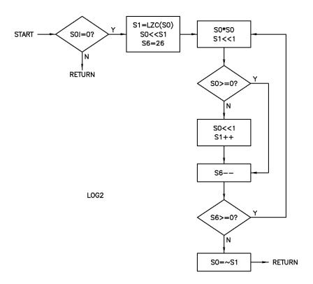
Figure 40. Log base 2 algorithm flow chart.
