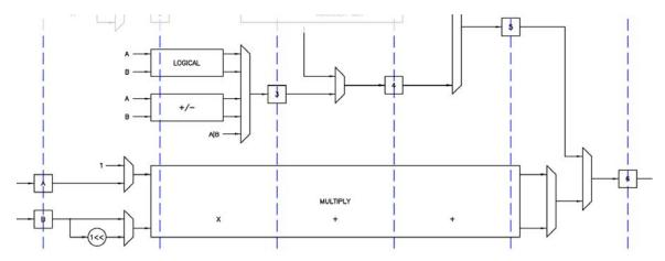
Figure 20. The Arithmetic and Logic Unit (ALU).
