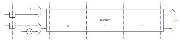
Figure 16. The Multiply and Shift unit.
