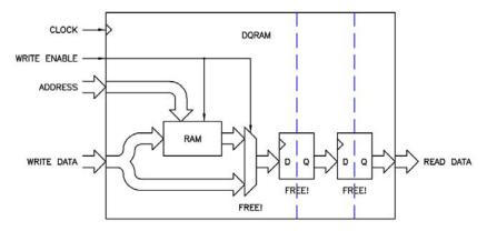
Figure 10. Block RAM internal resources.
