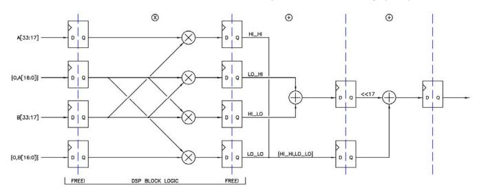
Figure 15. Three stage  $33 \times 33 = 66$  bit signed pipelined multiplication.
