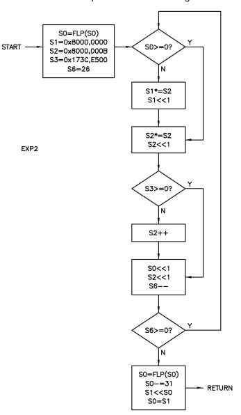
Figure 41. Exponential of 2 algorithm flow chart.
