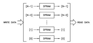
Figure 12. Block RAMs combined via bit-slice.
