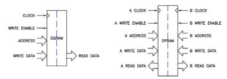
Figure 9. Block RAM: simple (DQ) on left, true dual port (DP) on right.
