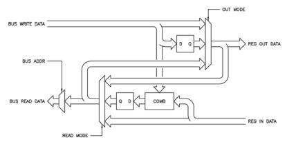
Figure 35. Configurable base register component.
