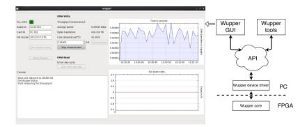
Figure 7: High and low level software overview block diagram.
