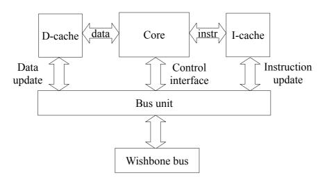
The bus unit connects the cache units via a pipelined Wishbone interface to the rest of the system. An example of a compatible Wishbone fabric can be found in the STORM\_core\_TB.vhd (sim folder). For more information about the Wishbone architecture, see the Wishbone data sheet in the doc folder.
