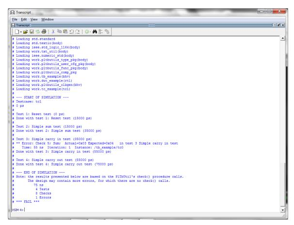
The transcript window clearly shows points in time where the simulation starts, ends, and where errors are detected. The simulation stops with a clear SUCCESS/FAIL message, specifically formatted for parsing by scripts.
