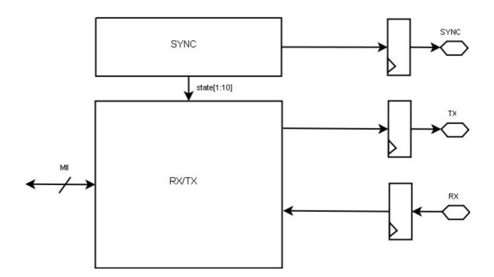
Instance SYNC can be used to multiple RX/TX modules. Use one RX/TX module per SMII channel. To ensure that DFFs on IO signals are placed in IO block a specific target module can be used. The exact module to use is target dependant. For target independent design there are two modules that can be used, OBUFDFF and IBUFDFF.
