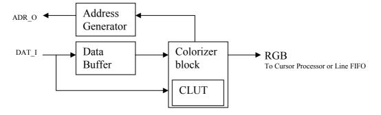
The Color Processor, together with the WISHBONE Master interface and the Line FIFO, handles the pixel color generation. The internal structure of the Color Processor, including parts of the WISHBONE Master interface, is shown in the figure above.
