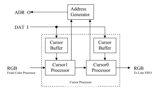
The Cursor Processor handles the hardware cursors together with the WISHBONE Master interface. The internal structure of the Cursor Processor, including parts of the WISHBONE Master interface is shown in the figure above. If a cursor is not implemented, it is a pass-through function. The above schematic still applies, but no logic is generated for that cursor.
