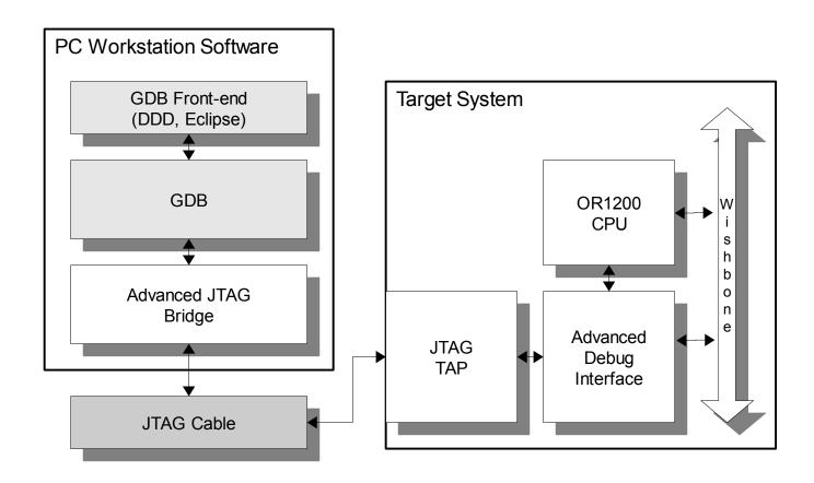
Figure 1: Debugging system block diagram
