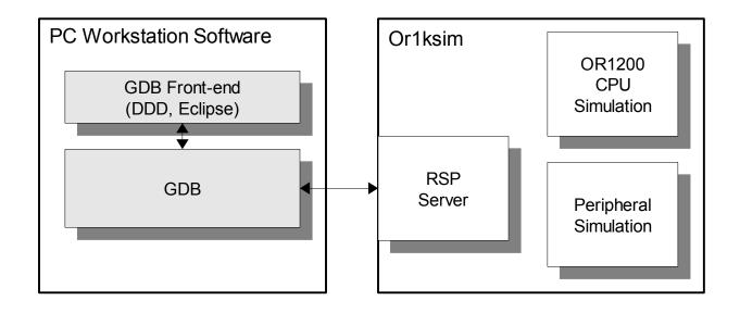
Figure 2: Block diagram of debugging system using or1ksim
