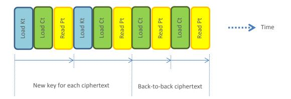
If a new ciphertext is loaded before the previous plaintext is read, the core will start to decrypt the new ciphetext immediately and the previous plaintext will be over-written. Loading a new key will only start a key expansion cycle internally and will not alter the previous plaintext.
