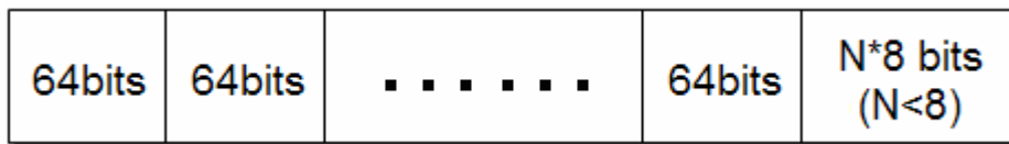
Figure 2-9 10Gigabit Ethernet Frame division
