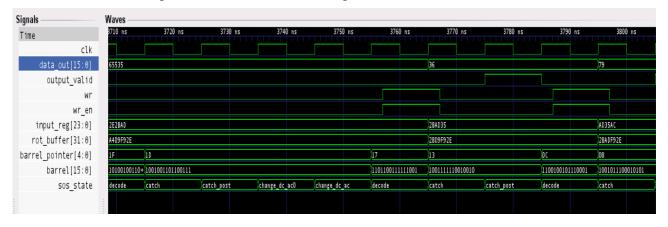
In this timing diagram you can see only some clocks are needed in this implementation. This is important for high value streaming like video applications.
