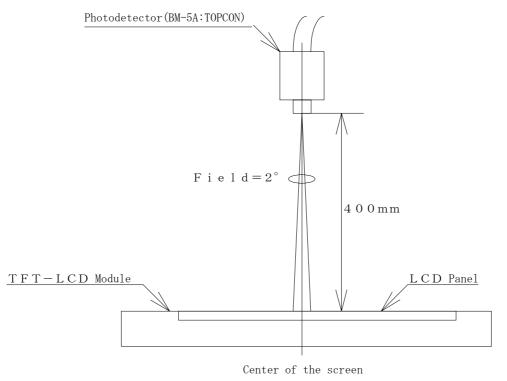
Optical characteristics measurement method
