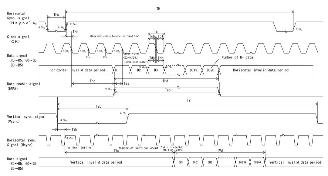
Fig.8 Input signal wave forms
