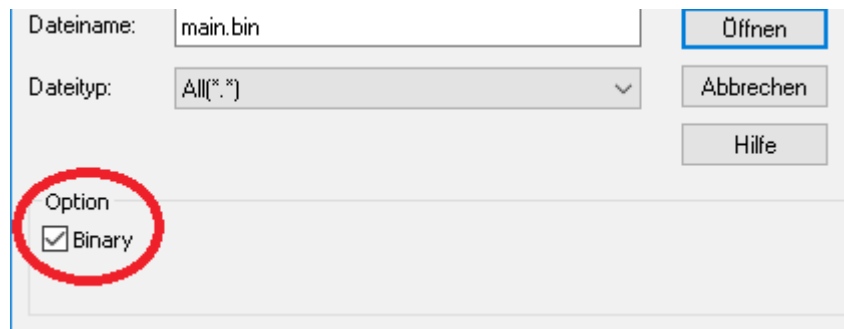
Figure 13: Transfer executable in binary mode (German version of TeraTerm)
