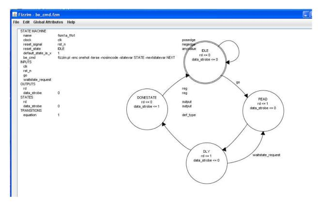
I can move the whole fsm by selecting all the states either by selecting each state individually (click, ctl-click, ctl-click, etc), or by drawing a box around the whole fsm:
