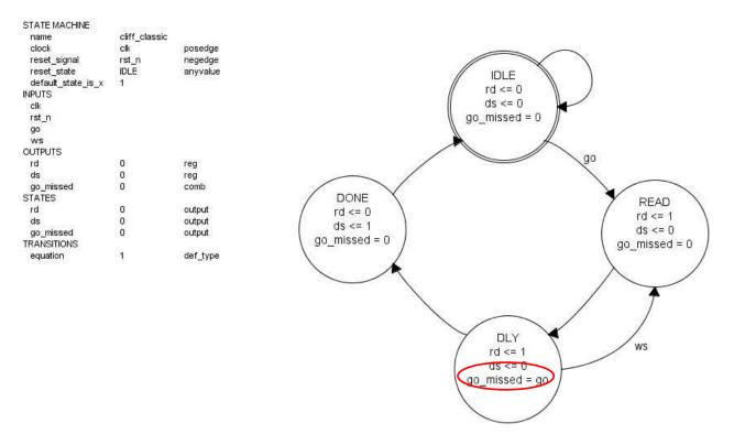
Notice the go\_missed output shows up on each state bubble with an "=" instead of a "<=", because it is of type "comb".
