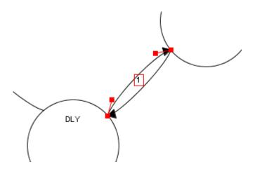
Drag the endpoints to a new location, then drag the anchorpoints to reshape the curve. The anchorpoints on the ends of the arc control where the arc intersects the state bubble. The other two control the shape of the curve.
