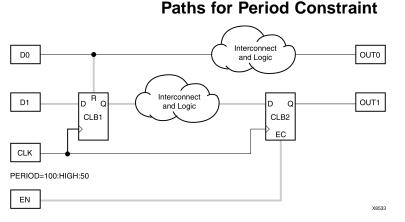
The timing tools do not check pad-to-register paths relative to setup requirements. For example, in the preceding figure, the path from **D1** to Pin **D** of **CLB1** is not included in the Period constraint. The same is true for **CLOCK\_TO\_OUT**.
