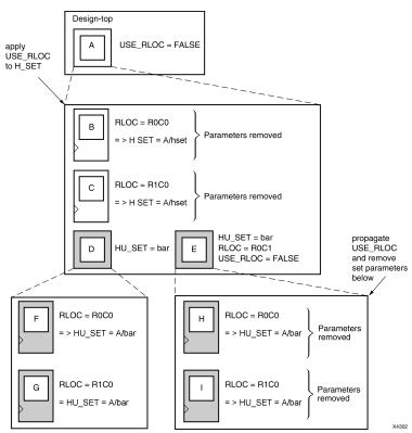
Applying the Use Relative Location constraint on U Set sets is a special case because of the lack of hierarchy in the U SET set. Because the Use Relative Location constraint propagates strictly in a hierarchical manner, the members of a U SET set that are in different parts of the design hierarchy must be tagged separately with the Use Relative Location constraint. No single Use Relative Location constraint is propagated to all the members of the set that lie in different parts of the hierarchy.
