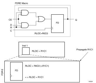
In this example, the RLOC = R1C1 constraint is attached to the instantiation (Inst1) of an example macro. It is added to the R0C0 value of the Relative Location constraint on the flip-flop within the macro to obtain the new RLOC values.
