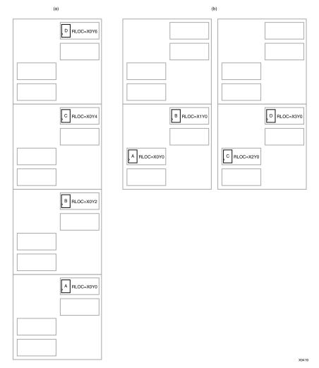
In diagram (a), four flip-flop primitives named A, B, C, and D are assigned Relative Location constraints. These Relative Location constraints require each flip-flop to be placed in a different slice with the slices stacked in the order shown: A below B, C, and D.
