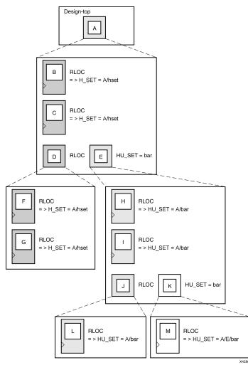
This example demonstrates how HU SET constraints designate elements as set members, break links between elements tagged with Relative Location constraints in the hierarchy to separate them from H SET sets, and generate names as identifiers of these sets.
