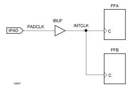
In the preceding design, a Timing Name constraint associated with the **IPAD** symbol includes only the **PAD** symbol as a member in a timing analysis group. For example, the following UCF file entry creates a time group that includes the **IPAD** symbol only.
