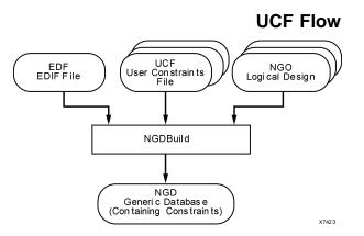
UCF files are input to NGDBuild (see the preceding figure). The constraints in the UCF files become part of the information in the NGD file produced by NGDBuild. For FPGA devices, some of these constraints are used when the design is mapped by MAP, and some of the constraints are written into the Physical Constraints File (PCF) produced by MAP.
