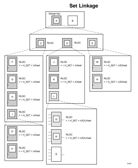
This example shows the process of linking together elements through the design hierarchy. The complete Relative Location specification, RLOC=R mCn or RLOC=XmXn, is required for a real design.
