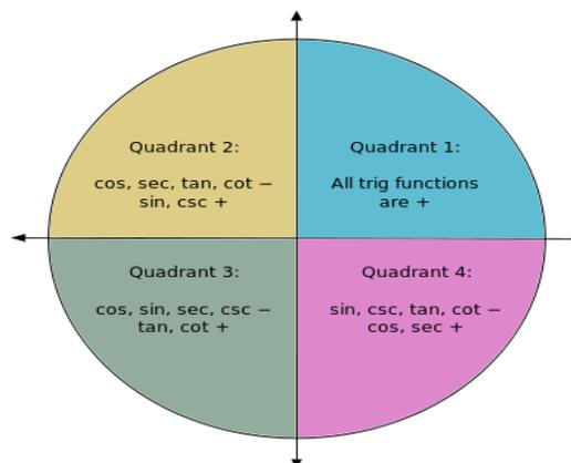
This architecture is created using look up table. But instead of creating the table for all the values it is created only for the first 90 values and all the remaining values are derived using these 90 values. From the top module using “ACTV” Input we can choose which function to activate.
