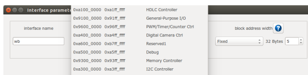
Figure 3.2: Slave WB address setting snapshot. The size of memory mapped registers in this example is 2^5 = 32 bytes. For a 32-width WB it is equal to 32/4 = 8 individual registers. In case, you have parameterizable number (e.g. M ) to indicate memory mapped register width in words in your IP module Verilog file, you need to add another parameter such as N=M+2 in parameter setting window and select its type as Don't include to be used as address width parameter in bytes.
