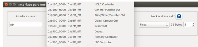
Figure 3.2: Slave WB address setting snapshot. The size of memory mapped registers in this example is 2^5 = 32 bytes. For a 32-width WB it is equal to 32/4 = 8 individual registers. In case, you have parameterizable number (e.g. M ) to indicate memory mapped register width in words in your IP module Verilog file, you need to add another parameter such as N=M+2 in parameter setting window and select its type as Don't include to be used as address width parameter in bytes.
