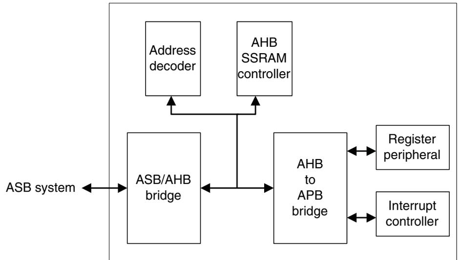
**Figure 6-2 Example with an ASB to AHB bridge**
