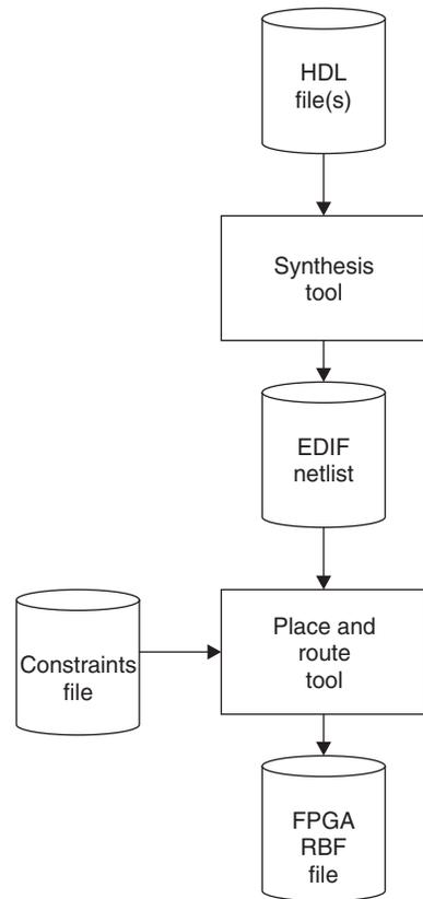
**Figure 4-2 Basic tool flow**
