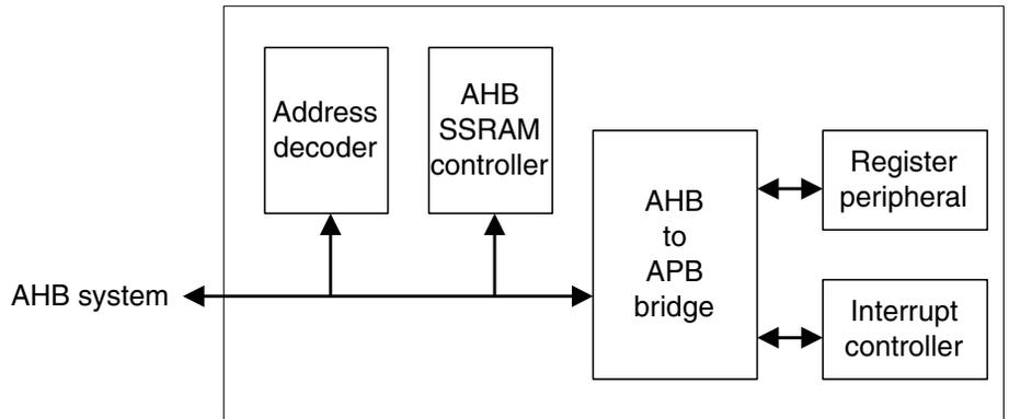
**Figure 6-1 Example without an ASB to AHB bridge**
