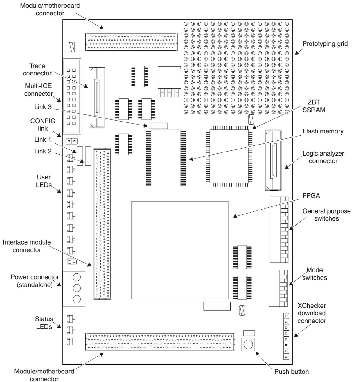
Figure 1-1 Integrator/LM-XCV600E+ layout
