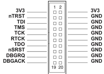
Figure A-6 Multi-ICE connector pinout
