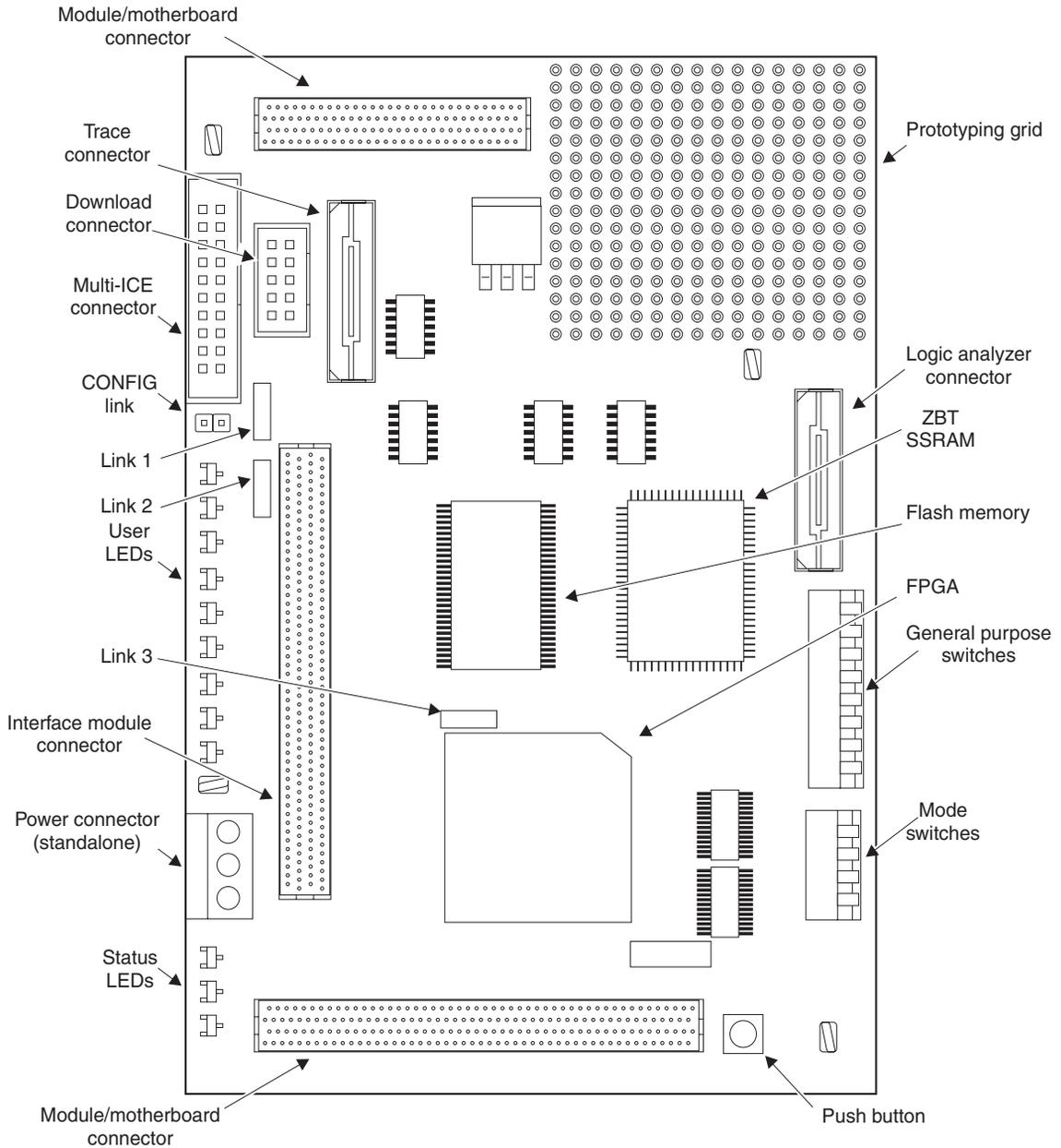
Figure 1-2 Integrator/LM-EP20K600E+ layout
