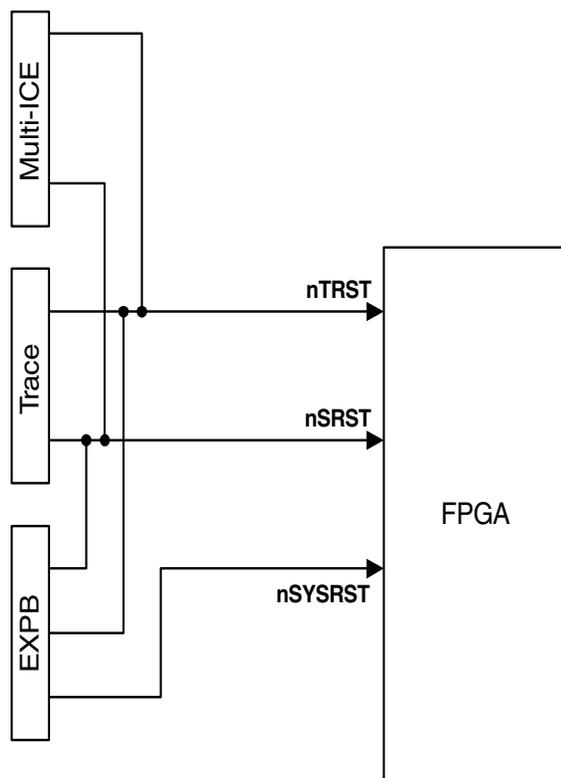
Figure 3-2 Reset architecture
