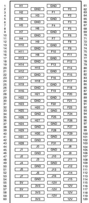
Figure A-3 EXPB plug pin numbering
