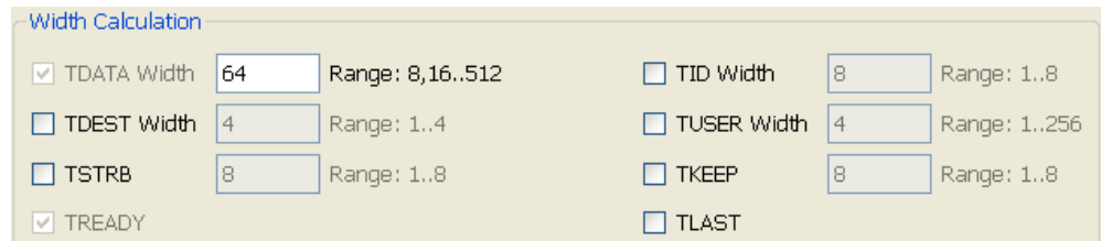
Figure 8-6: AXI4 Interface FIFO: Page 3 - Write Width Calculation
