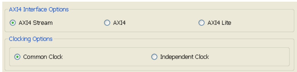
Figure 8-3: AXI4 Interface FIFO: Page 2 - Interface and Clocking Options
