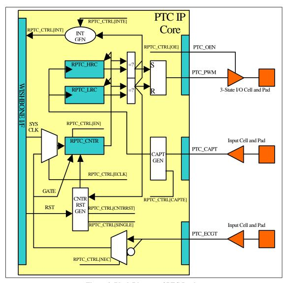
Figure 2. Block Diagram of PTC Logic
