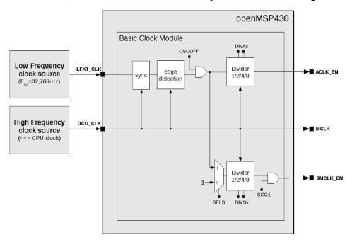
**Note**: CPUOFF doesn't switch MCLK off and will instead bring the CPU state machines in an IDLE state while MCLK will still be running.
