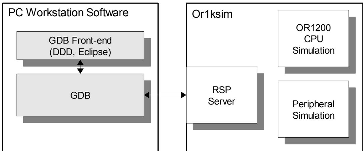
Figure 2: Block diagram of debugging system using or1ksim
