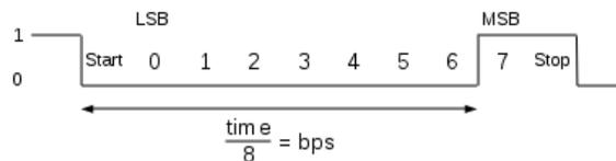
As you can see, the host simply sends the 0x80 value. The openMSP430 will then measure the time between the falling and rising edge, divide it by 8 and automatically deduce the baud rate it should use to properly communicate with the host.
