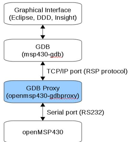
Like the original '*msp430-gdbproxy*' program, '*openmsp430-gdbproxy*' can be controlled from the command line. However, it also provides a small graphical interface:
