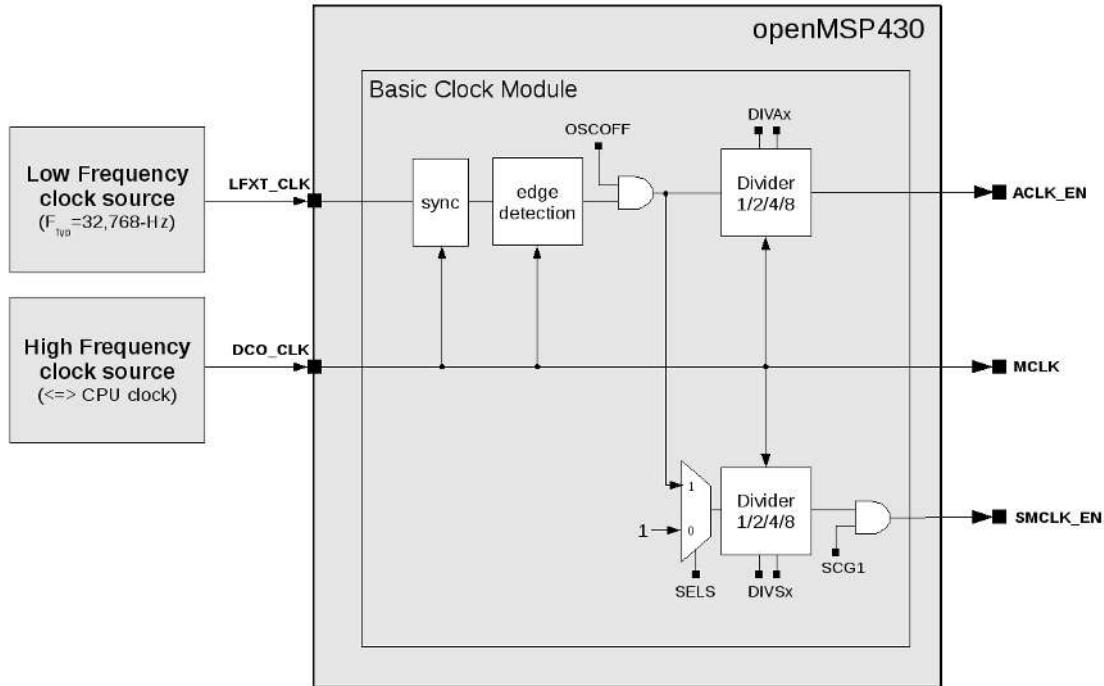
**Note:** CPUOFF doesn't switch MCLK off and will instead bring the CPU state machines in an IDLE state while MCLK will still be running.
