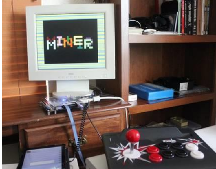
Image 3 : Sinclair ZX Spectrum on Altera DE1
