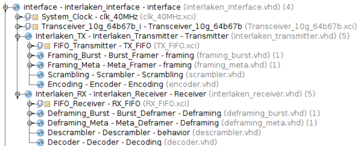
Figure 44: Structure of the project in Vivado
