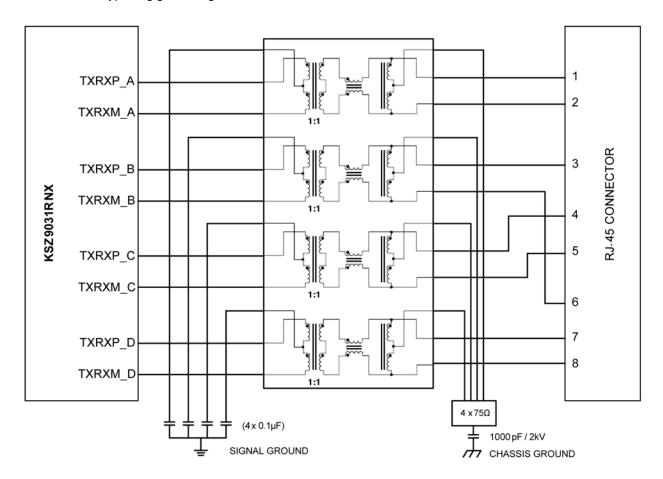
Figure 20. Typical Gigabit Magnetic Interface Circuit
