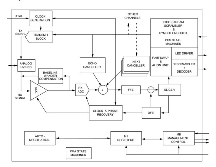
Figure 2. KSZ9031RNX 1000Base-T Transceiver Block Diagram - Single Channel
