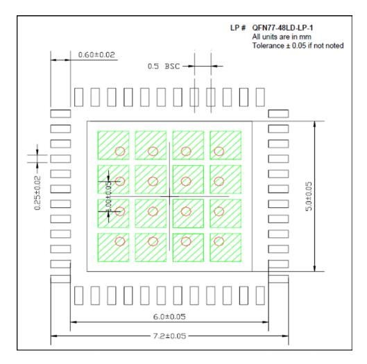
Red circles indicate thermal vias. They should be 0.350mm in diameter and be connected to the GND plane for maximum thermal performance.
