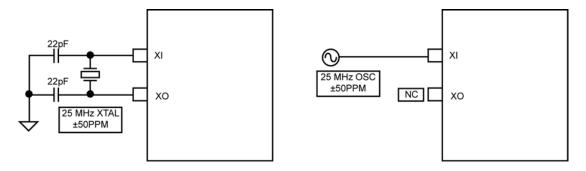
Figure 19. 25MHz Crystal/Oscillator Reference Clock Connection
