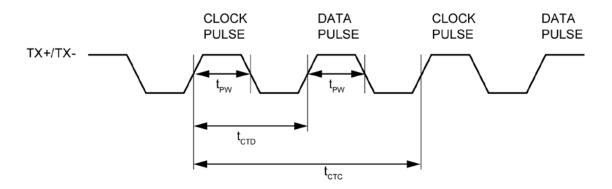
Figure 13. Auto-Negotiation Fast Link Pulse (FLP) Timing
