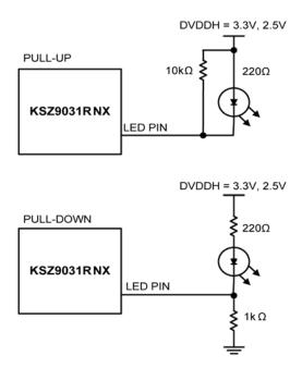
Figure 18. Reference Circuits for LED Strapping Pins
