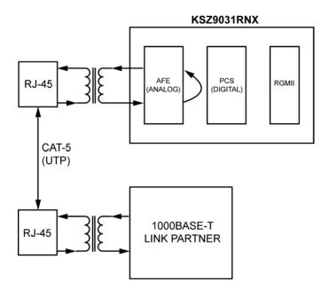
Figure 6. Remote (Analog) Loopback
