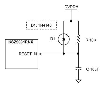
Figure 16. Recommended Reset Circuit
