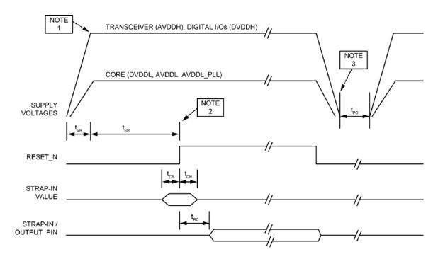
Figure 15. Power-Up/Power-Down/Reset Timing
