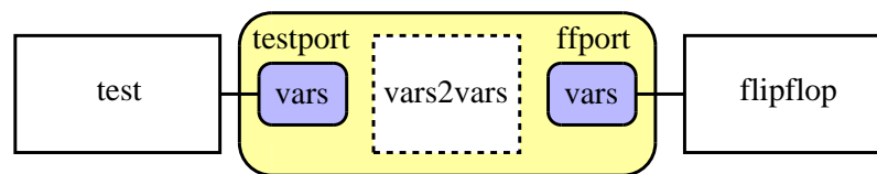
Figure 5: Outline of interfacing two vars ports
