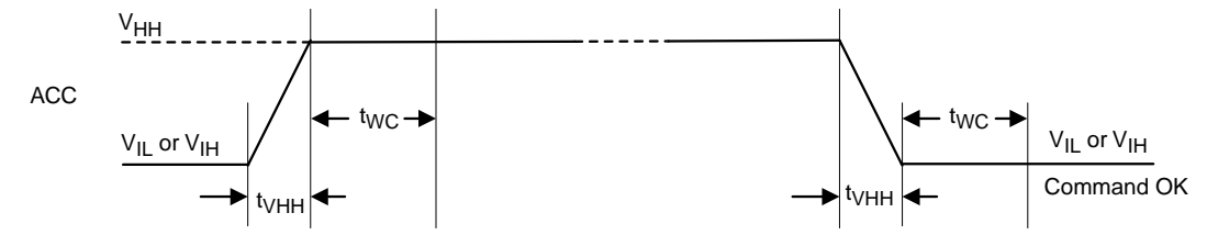
Figure 13.1 ACC Program Acceleration Timing Requirements
