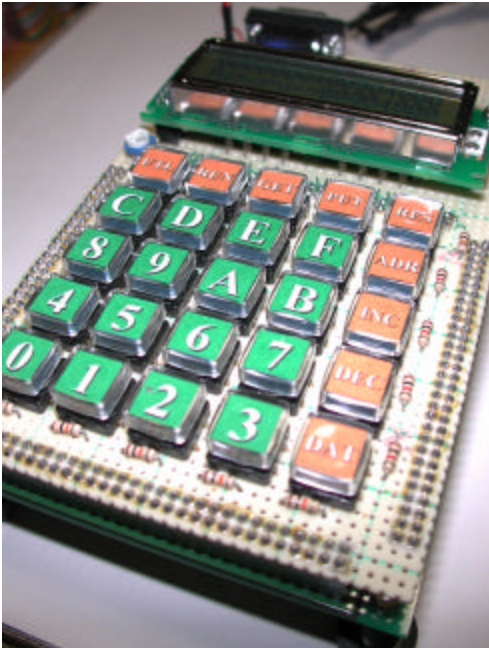
Figure7.1 FPGA Verification System
