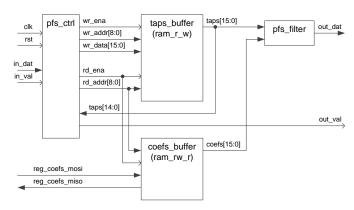
Figure 4 Architecture single channel poly phase filter
