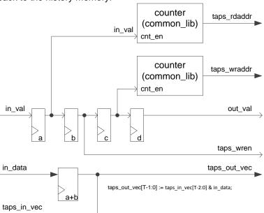
Figure 8 Detailed block diagram of fil ppf ctrl
