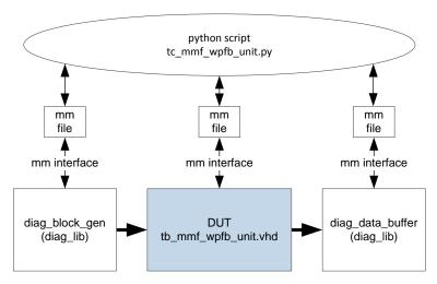
Figure 10 Testbench based on co-similulation
