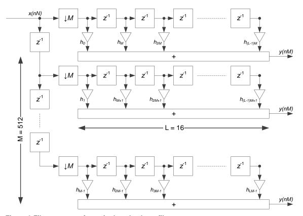
Figure 3 Filter structure for a single poly phase filter
