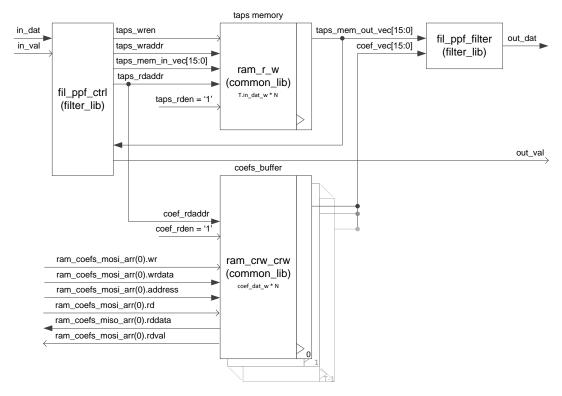
Figure 6 Detailed block diagram of fil\_ppf\_single
