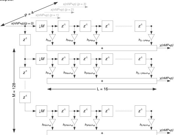
Figure 5 Filter structure for a wideband poly phase filter
