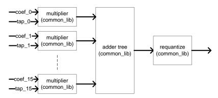
Figure 7 Block diagram of the ppf\_filter unit
