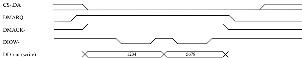
Figure 4.7 32bit DMA write transfer, without endian conversion
