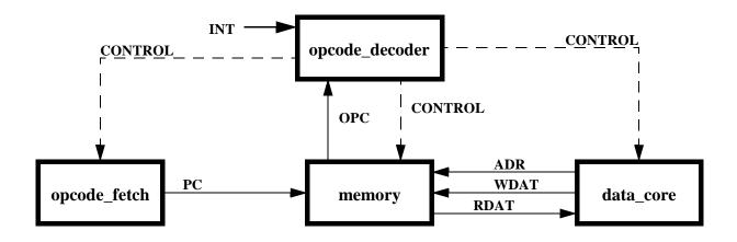
The memory signals are also extended to the outside of this module in order to connect to an optional external SRAM and to the **input\_output.vhd** module.
