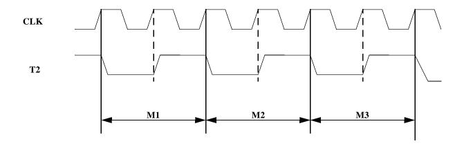
We call a full T2 cycle an M cycle; most opcodes use only a single M cycle (M1), opcodes with a short immediate operand require two M cycles (M1 and M2), and so on. The longest opcode is RET, reading the return address in M2 and M3, plus 2 M cycles delay from the PC to the excution unit.
