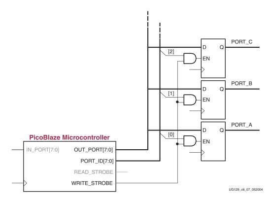
Figure 6-7: Simple Address Decoding for Designs with Few Output Destinations
