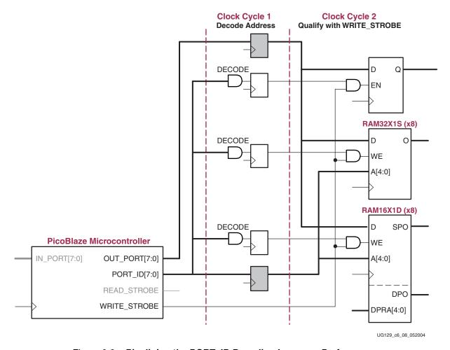
Figure 6-9: Pipelining the PORT\_ID Decoding Improves Performance
