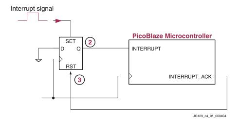
Figure 4-1: Simple Interrupt Logic
