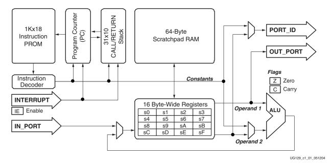
Figure 1-1: PicoBlaze Embedded Microcontroller Block Diagram
