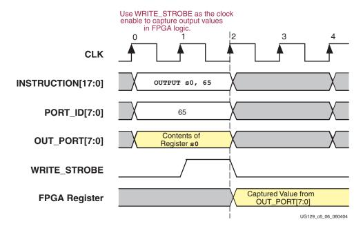
Figure 6-6: Port Timing for OUTPUT Instruction
