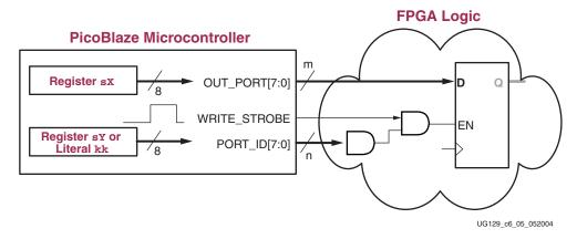
Figure C-7: OUTPUT Operation and FPGA Interface Logic
