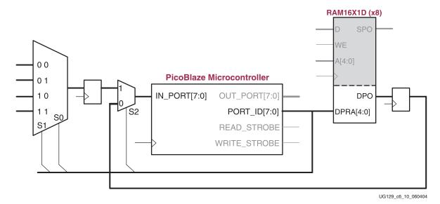
Figure 6-11: Effective Pipelining Improves Read Performance
