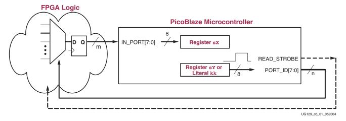
Figure 6-1: INPUT Operation and FPGA Interface Logic
