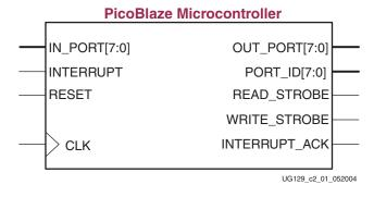
Figure 2-1: PicoBlaze Interface Connections
