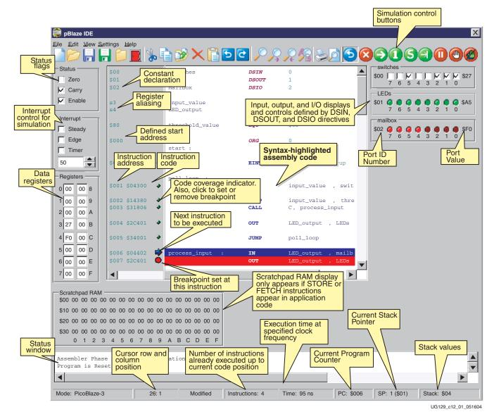
Figure 12-1: The pBlazIDE Instruction Set Simulator (ISS)
