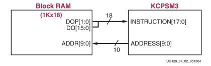
Figure 7-2: Standard Configuration using a Single 1Kx18 Block RAM
