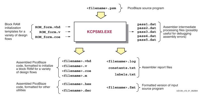
Figure 10-1: KCPSM3 Assembler Files
