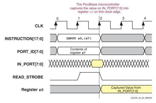
Figure 6-2: Port Timing for INPUT Instruction
