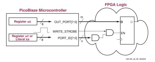
Figure 6-5: OUTPUT Operation and FPGA Interface
