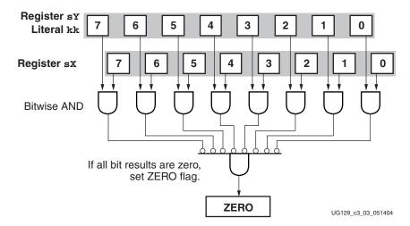
Figure C-11: ZERO Flag Logic for TEST Instruction
