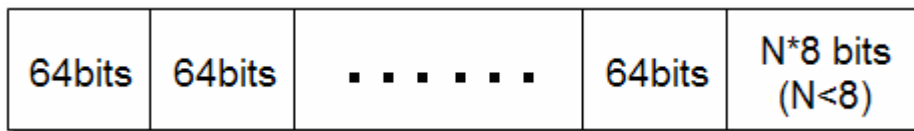
Figure 2-9 10Gigabit Ethernet Frame division
