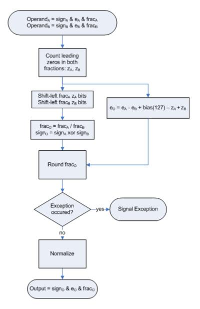
The division was done serially using the basic algorithm taught in most schools, which is division through multiple subtractions. Since divisions are not needed as often as multiplications (divisions can be done also through multiplications!), it was implemented as serial and in the process saving some hardware area.
