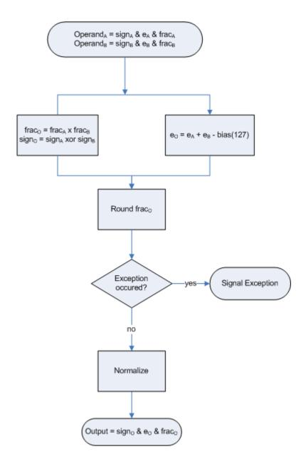
The multiplication was done parallel to save clock cycles, at the cost of hardware. If done serial it would have taken 32 clock cycles (without pre-, post-normalization) instead of the actual 5 clock cycles needed. Disadvantage, the hardware needed for the parallel 32-bit multiplier is approximately 3 times that of serial.
