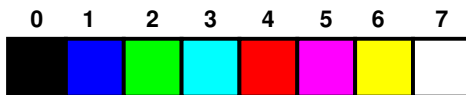
Figure 3.1: The color palette as used by the VGA controller. The numbers above the colors indicate the index for the foreground or background color.
