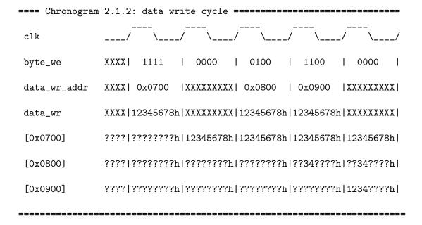
Note the two back-to-back stores to addresses 0x0800 and 0x0900. They are produced by two consecutive S\* instructions (SB and SH in the example), and can only be done this fast because of the Harvard architecture (and, again, because the diagram does not account for the cache interaction).
