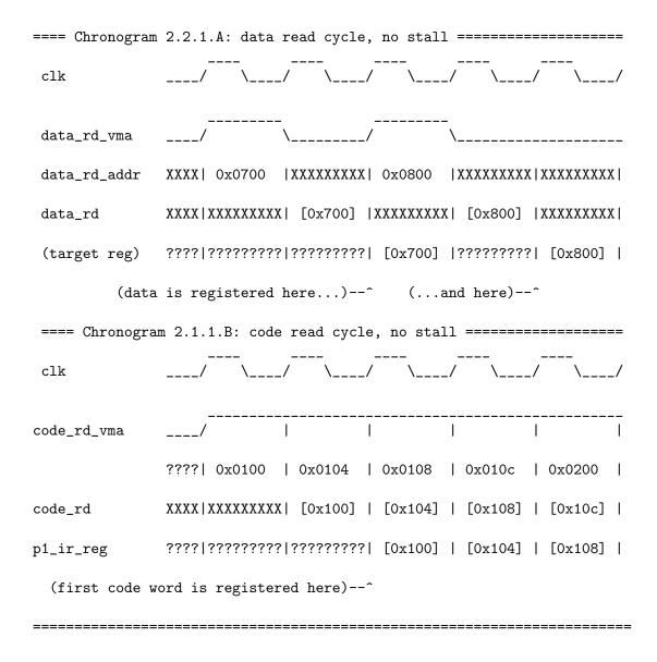
The data address bus is 32-bit wide; the lowest 2 bits are redundant in read cycles since the CPU always reads full words, but they may be useful for debugging.
