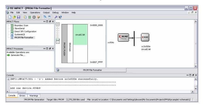
Under the iMPACT Processes panel, double-click the Generate File... option. iMPACT creates the .mcs file along with several other files. These other files can be ignored. The .mcs file is used by the Adept application or iMPACT to configure the platform flash on a Digilent system board.
