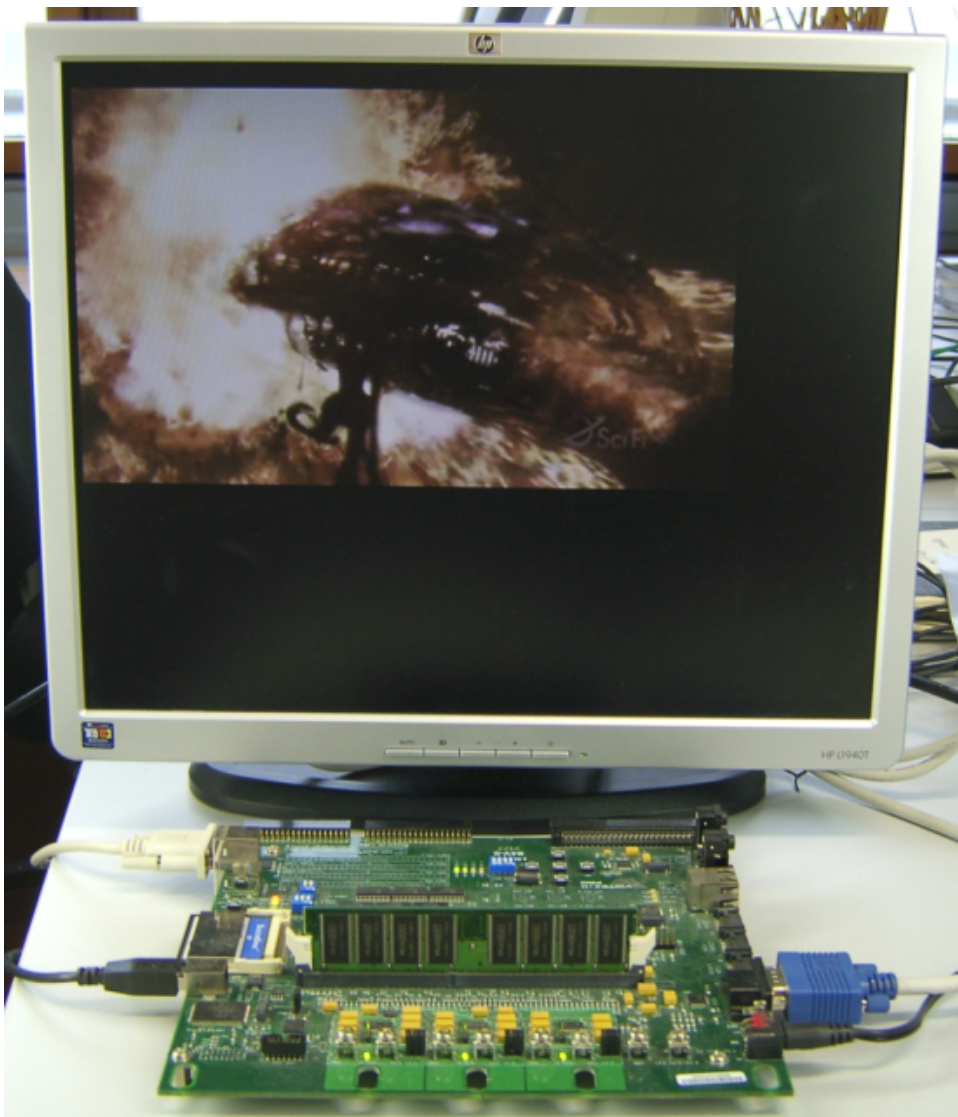
Figure 6.7: The Xilinx XUP Virtex-II Pro Development System board decoding an MotionJPEG movie and displaying it on a VGA monitor.
