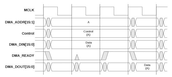
For both read and write operations the DMA master must hold the address, control and write data stable throughout the extended cycles.
