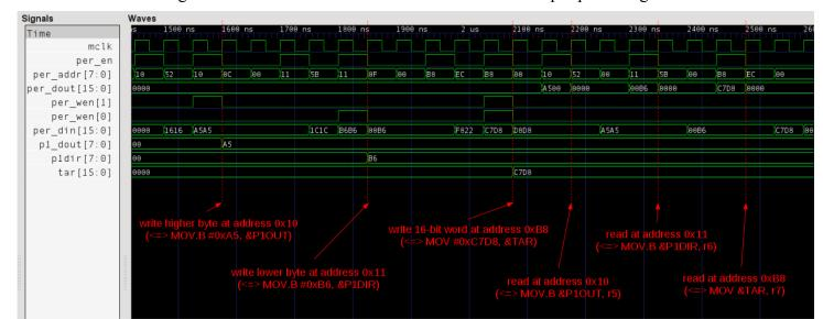
The following waveform illustrates some read/write access to the peripheral registers:
