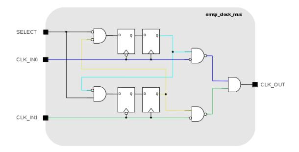
In order to make this implementation 100% bullet proof, the RTL could be modified by manually instantiating the NAND2 and AND2 cells directly from the target library (with the associated *don't touch* or *size only* attributes of course).
