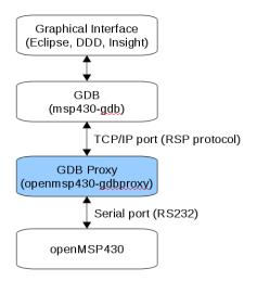
Like the original '*msp430-gdbproxy*' program, '*openmsp430-gdbproxy*' can be controlled from the command line. However, it also provides a simple graphical interface:
