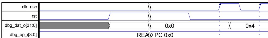
Figure 5. Power-Up and Reset Sequence w/ Gated Clock
