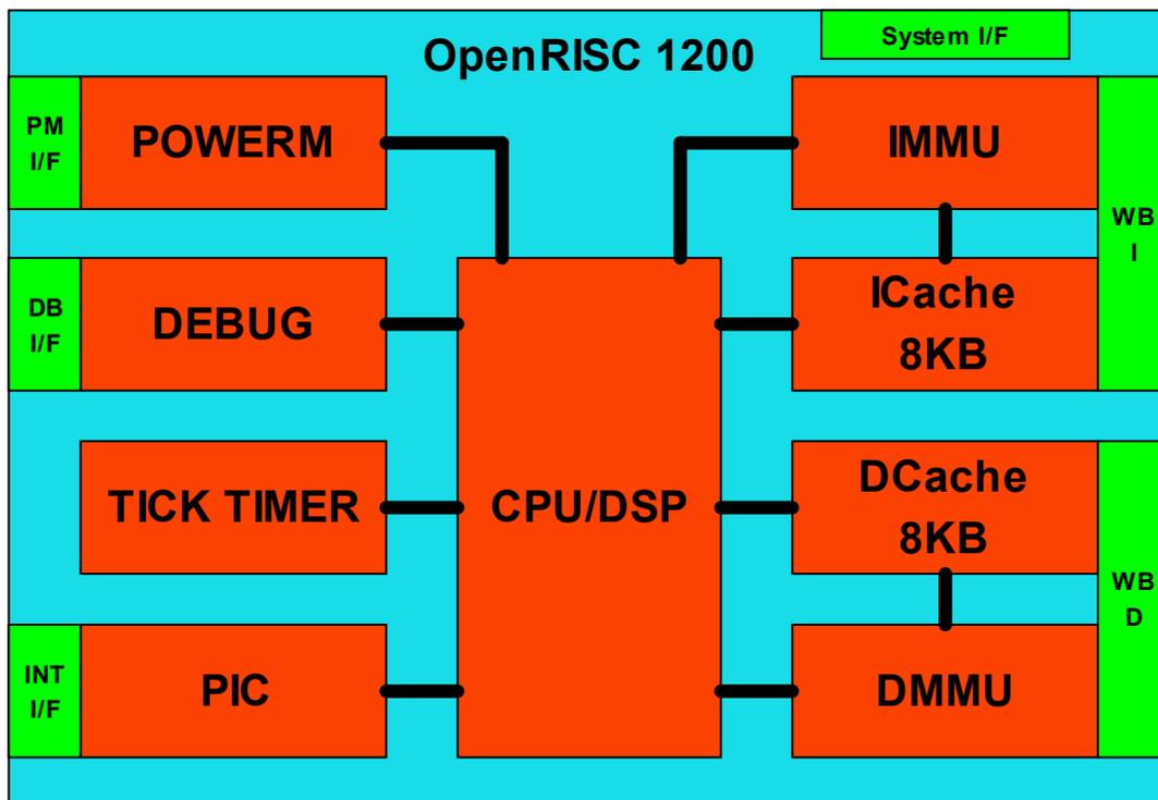
Figure 1. Core's Architecture
