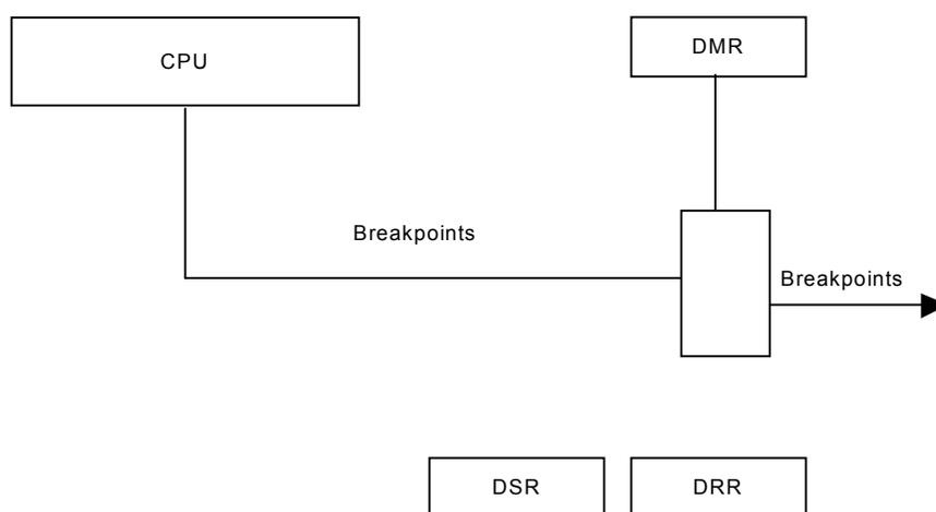
**Figure 3. Block Diagram of Debug Unit**
