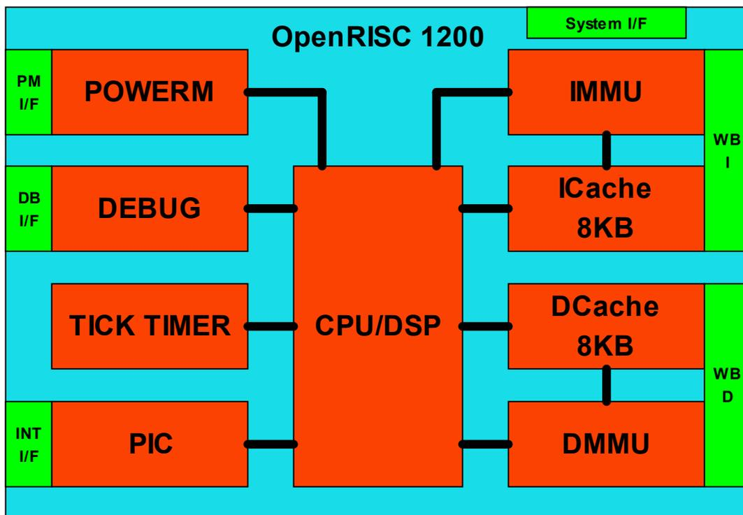
Figure 14. Core's Interfaces
