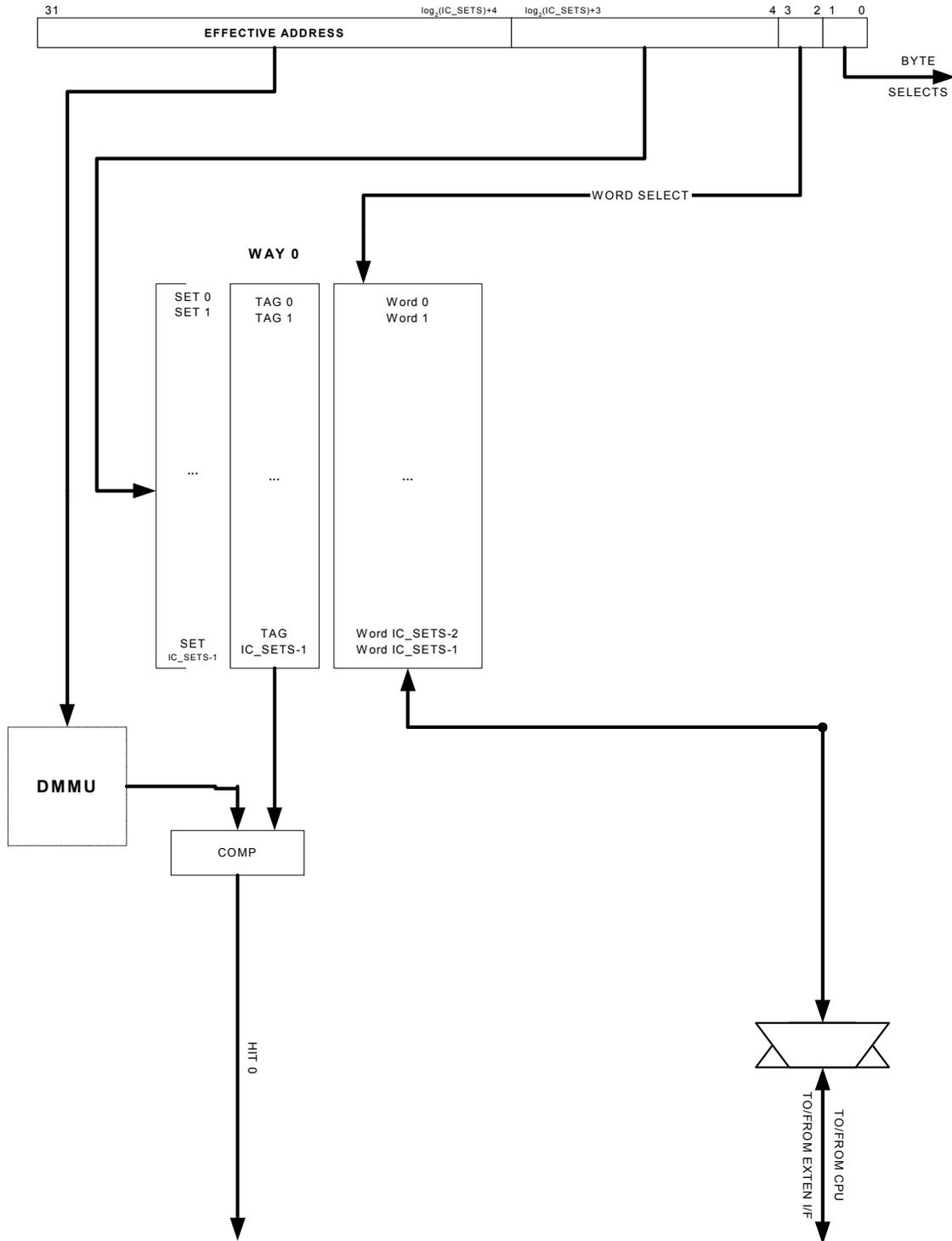
Each line contains four contiguous words from memory that are loaded from a four-word aligned boundary. As a result, cache lines are aligned with page boundaries.
