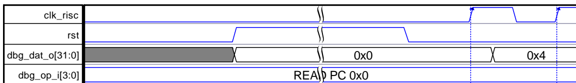
Figure 5. Power-Up and Reset Sequence w/ Gated Clock
