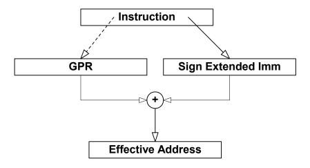
Figure 3-1. Register Indirect with Displacement Addressing
