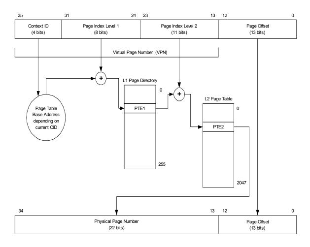
Figure 8-3. Address Translation Mechanism using Two-Level Page Table
