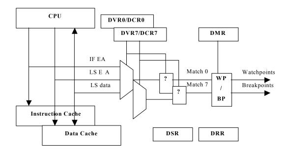
Figure 10-1. Block Diagram of Debug Support
