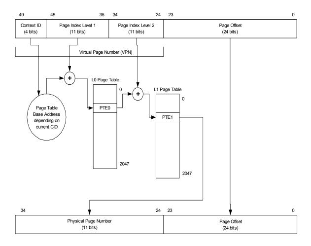
Figure 8-7. Address Translation Mechanism using Two-Level Page Table
