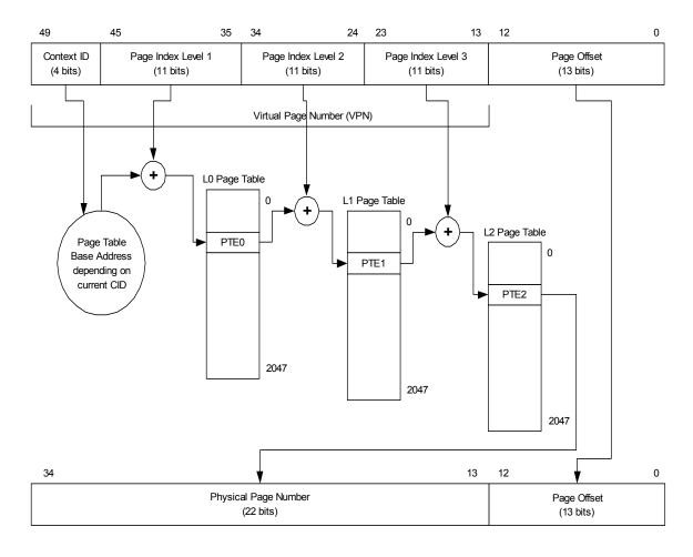
Figure 8-6. Address Translation Mechanism using Three-Level Page Table
