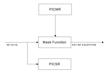
Figure 13-1. Programmable Interrupt Controller Block Diagram
