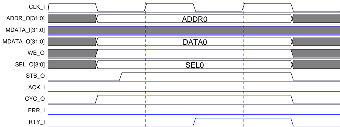
Figure 6-22: Retry on WISHBONE bus caused by PCI to WISHBONE transfer
