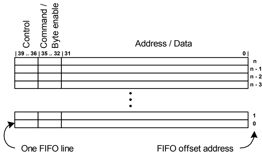
Figure 2-4: Detailed description of FIFO register lines
